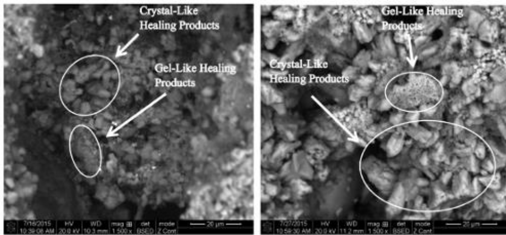
Figure 9: Healing Products in the Mortar Specimen Crack (Control: Left, 1% Microcapsule Content, Right)
