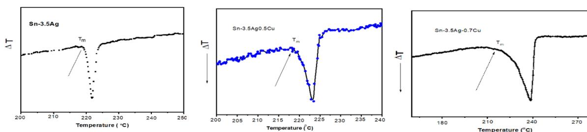
The area beneath the DTA peak and the calibration curve of the DTA, with Tin as a reference, were used to estimate the experimental evaluation of the enthalpy ( $\Delta H$ ) during the melting process ( $\Delta H_{ref}$ ). Once the formula is applied:
