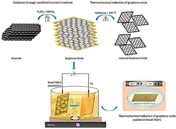
Electrophoretic deposition of GO on basalt fabric
